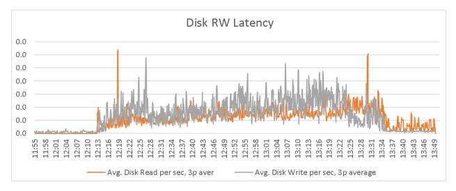
The graph below shows disk transfer metrics. For the Office Worker workload, disk transfers during steady state averaged about 134 IOPS for the test group of 77 users, or about 1.74 IOPS per Office Worker user. The peak value was 468 IOPS for 77 users or about 6.1 IOPS per Office Worker user. Disk transfer activity is also visible during the logoff period as user profile data is recorded.
