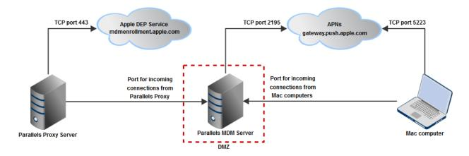
Please note that ports which numbers are specified on the diagram are used to communicate with Apple services and cannot be changed. Port numbers that are not specified (the Parallels MDM Server ports) are configured when you run the Parallels MDM Server Configuration Wizard. Please also see the table below for the list of ports shown on the diagram. All of these ports must be opened for communication.
