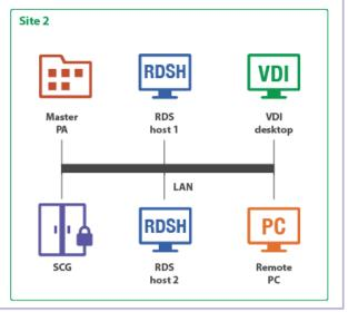
Adding more RAS Publishing Agents and RAS Secure Client Gateways adds redundancy to the system. HALB is an optional component, which can be added to load balance application traffic.
