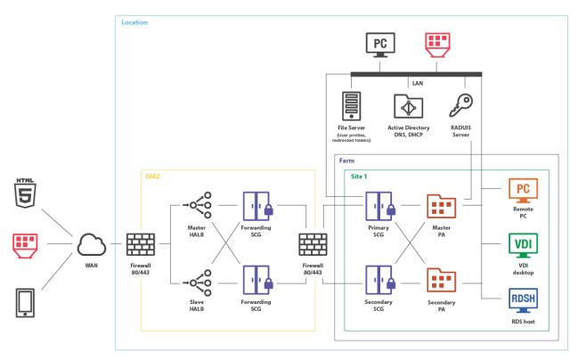
In a configuration of this type the second-level authentication via a RADIUS server is performed first. If the authentication procedure is successful, the next authentication takes place at the Active Directory level using either a user name and password or a smart card.
