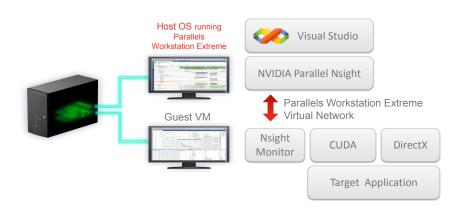
Now, Parallels Workstation Extreme addresses this problem, enabling developers to run both the host and target machines together on one Intel Xeon-based workstation, each with its own dedicated GPU. Parallels Workstation Extreme is a powerful, next-generation virtualization platform that gives end-users dedicated graphics and networking resources for both host and guest workstation environments.
